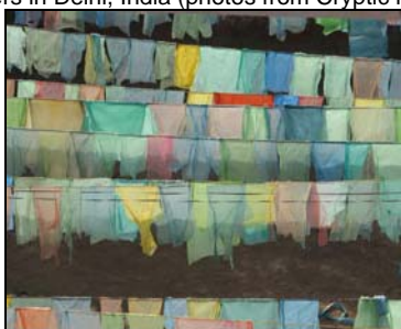
Plastic bags drying in the sun before conversion into woven fabric.
